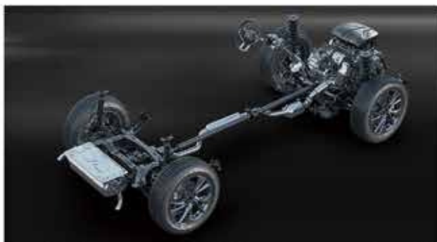
Front Macpherson rear multi-link independent suspension + AWD
